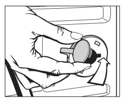
Fit the covers on to the two holes. Then plug the holes as shown with the caps. A The washing machine must not be moved without the transit bars in place.
